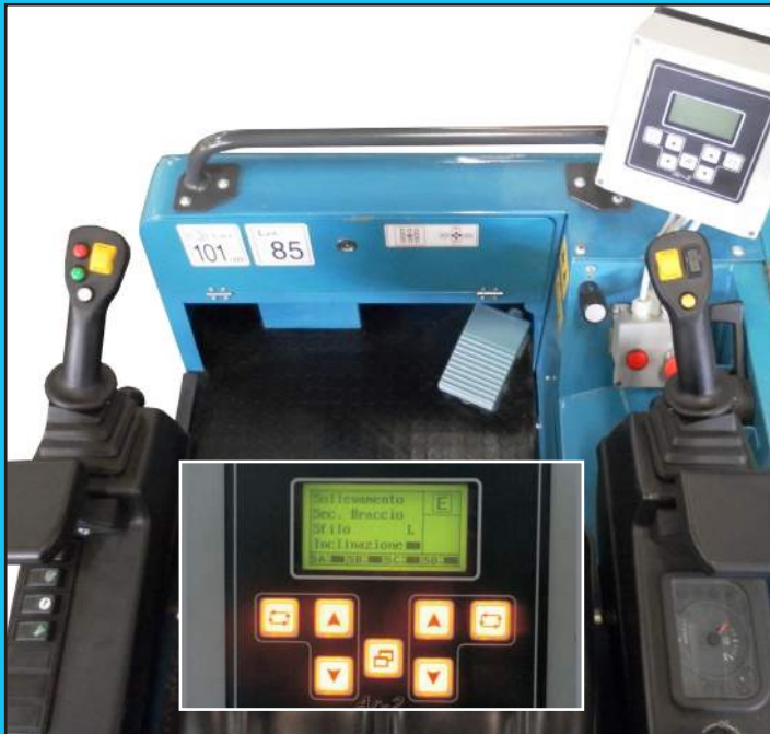
Machine driven with dual joy-sticks, left for traction and right for boom control.
